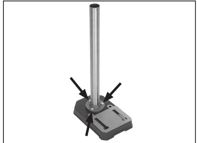
Figure 5. Column secured to base.
